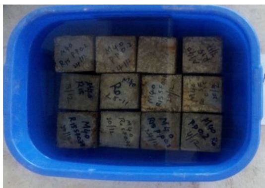
Fig. 20 Specimens immersed in artificial marine water
