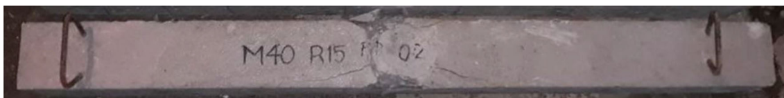
Fig. 24 Crushing at the top of the beam (typical)
