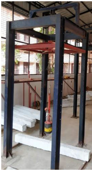
Fig. 12 Drop-weight test on beams
