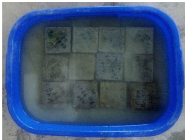
Fig. 21 Specimens immersed in acid
