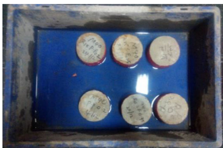
Fig. 19 Sorptivity testing on cylinders
