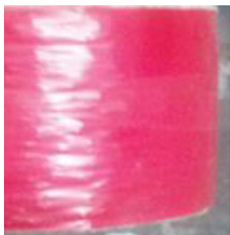
Fig. 18 Specimen wrapped in nonabsorbent filament around concrete cylinders
