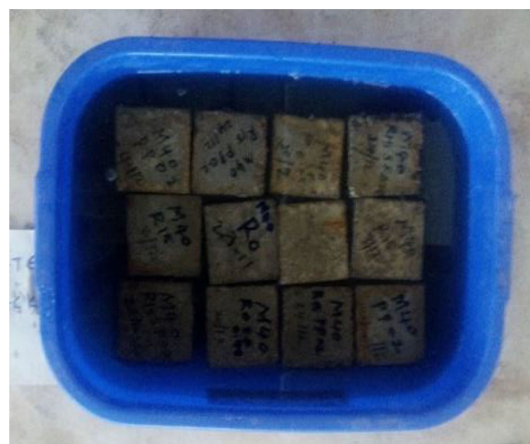
Fig. 22 Specimens immersed in sulphate solution
