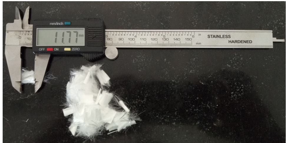
Fig. 2 Image showing discrete polypropylene fiber
