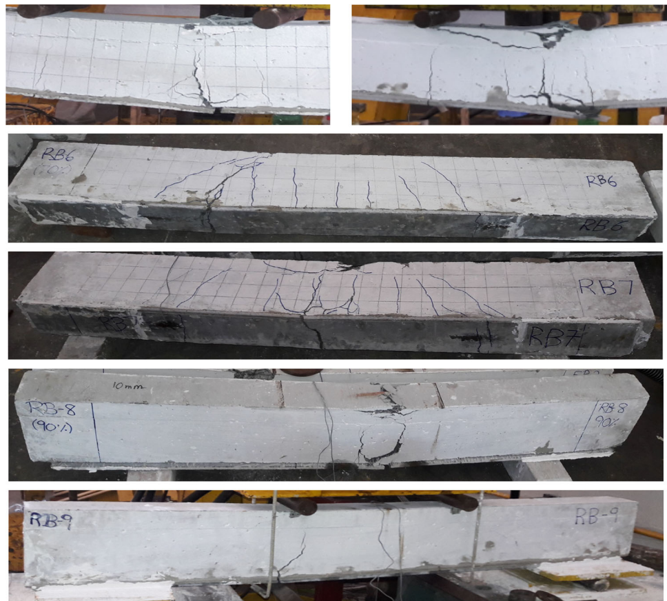
Fig. 6 Typical bonding of UHPFRC on NSC beams after failure
