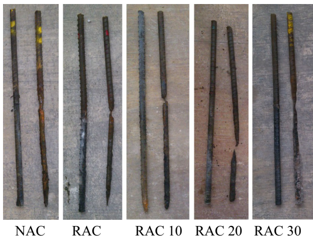
Fig. 16 Corroded rebars taken out from specimens of linear polarization test
