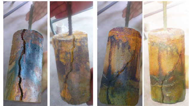
Fig. 14 Damaged specimens with rebars after impressed voltage test
