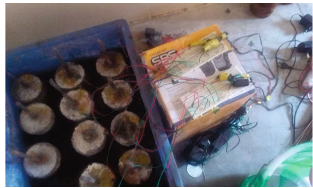
Fig. 7 Experimental setup for impressed voltage test
