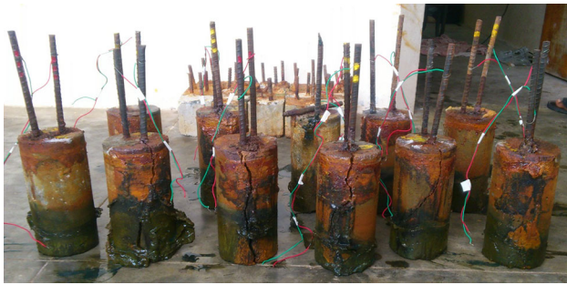
Fig. 11 Damaged specimens with rebars after linear polarisation test
