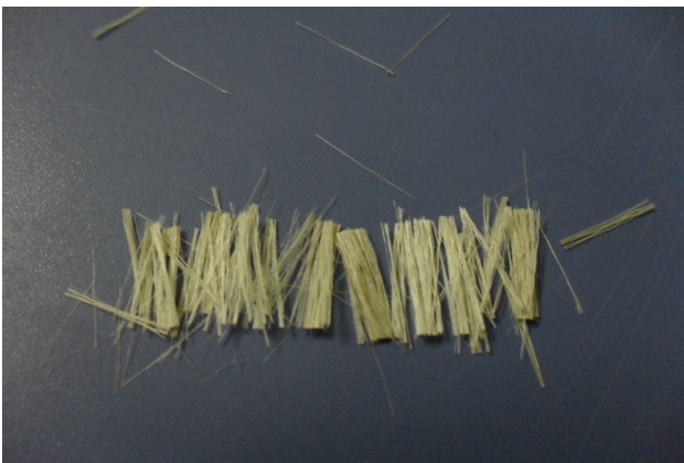
Fig. 2 Jute fiber cut into pieces of definite length
