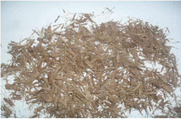
Fig. 1 Coir fiber cut into pieces of definite length
