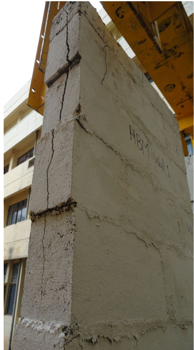
Fig. 11 Lateral splitting of HCB-150-A-7
