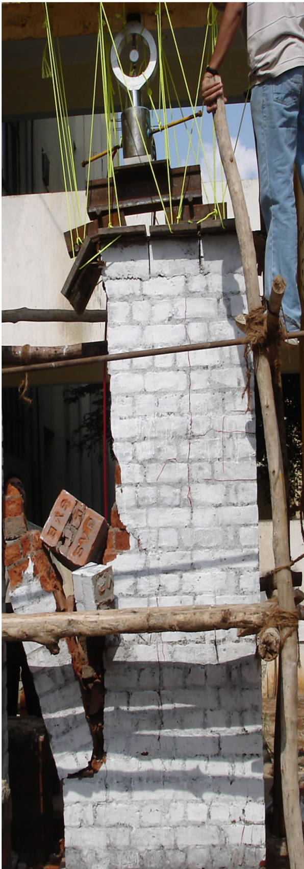
◀ Fig. 7 Vertical separation in TMB-230-A-3
