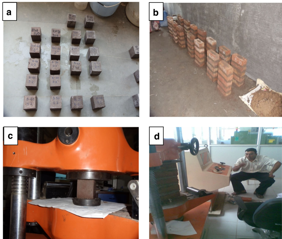
Fig. 1 a Mortar cube, b clay brick masonry prism, c compressive strength of mortar cube and d compressive strength of prism under UTM
