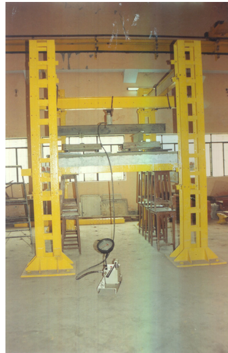
Fig. 5 Ferrocement slab panel under test
