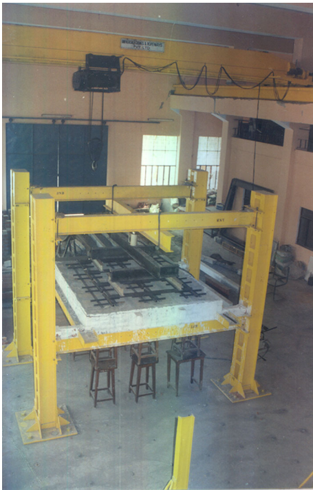
Fig. 3 Loading arrangement on slab panels
