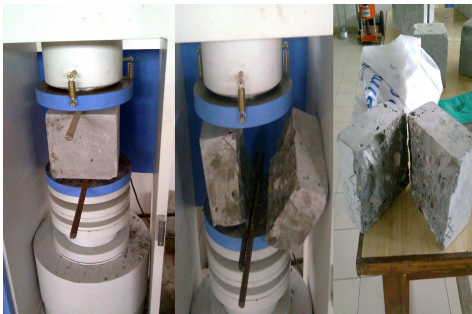
Fig. 5 Method to determine the bond strength of FGM cube
