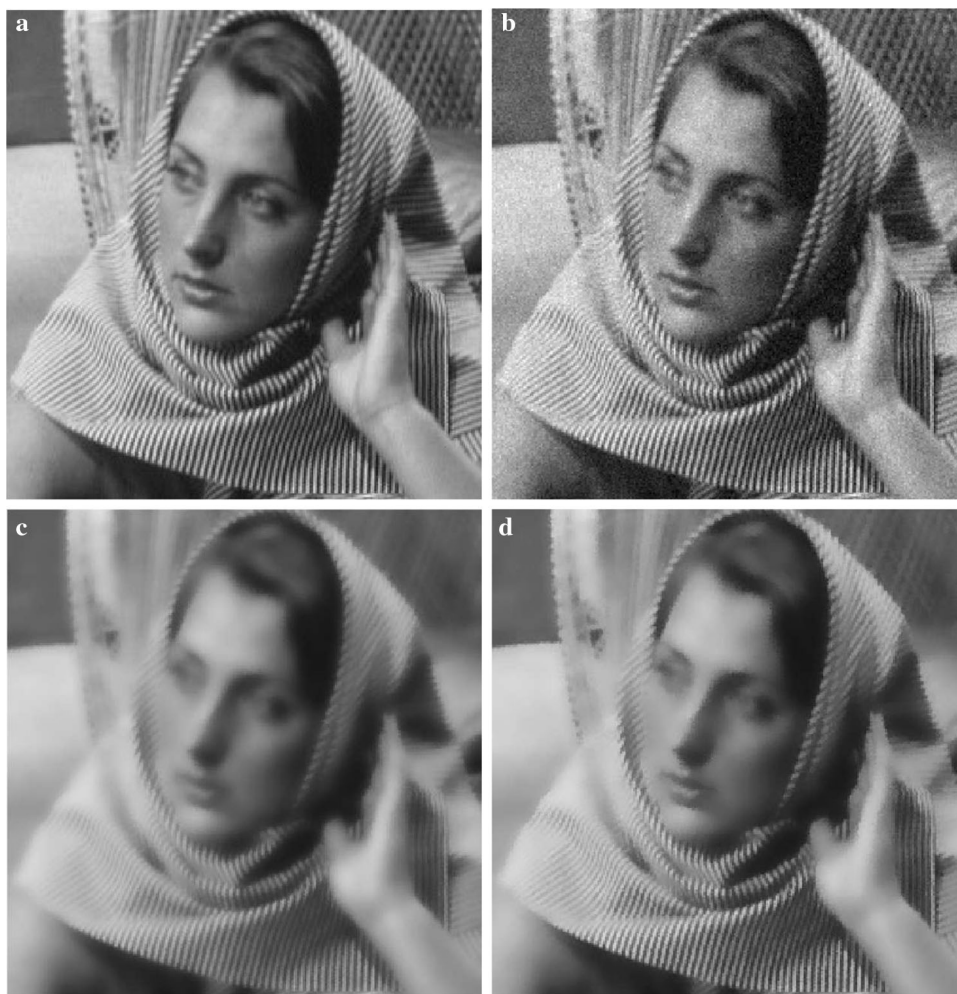
Fig. 1 a Input image (Barbara), b noisy image ( \sigma = 10 ), c bilateral filtered image (PSNR = 24.29 dB), d proposed texture and edge preserved Bilateral filtered image (PSNR = 27.09 dB)
