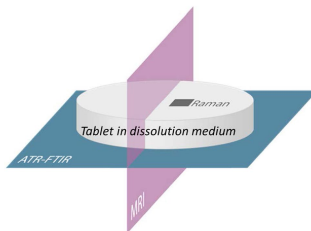
Fig. 5 Scheme of image position relative to the tablet, provided by each imaging method. Adapted from reference (Punčochová et al. 2016)
