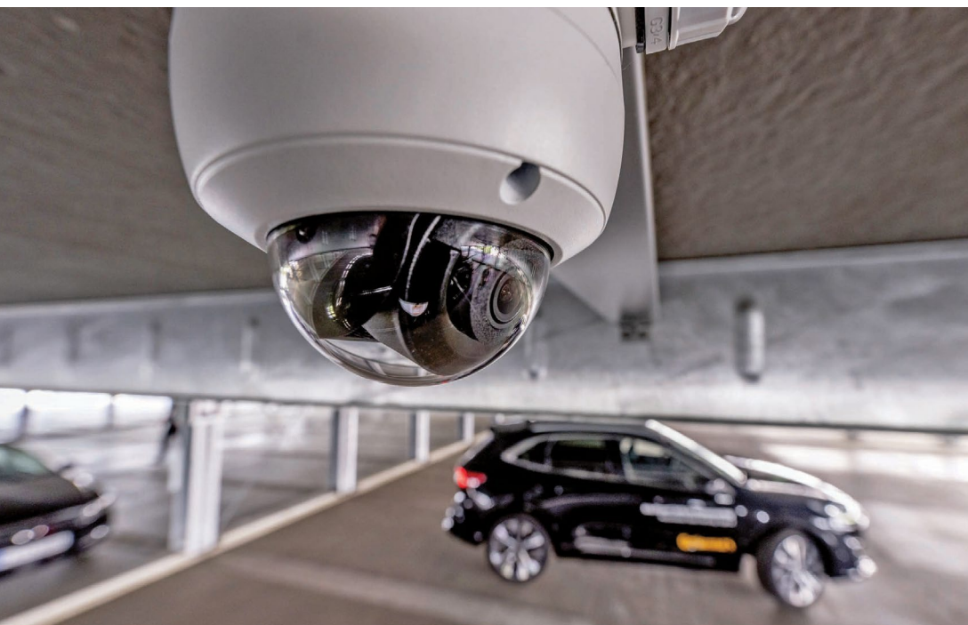
FIGURE 3 Standard surveillance cameras serve as main data source for vehicle localization and object perception (© Continental)
