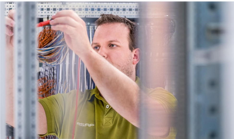
FIGURE 1 Lines of communication between all control units in the test system must be wired correctly (© ASAP Group)
