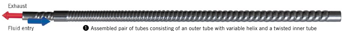
1 Assembled pair of tubes consisting of an outer tube with variable helix and a twisted inner tube
