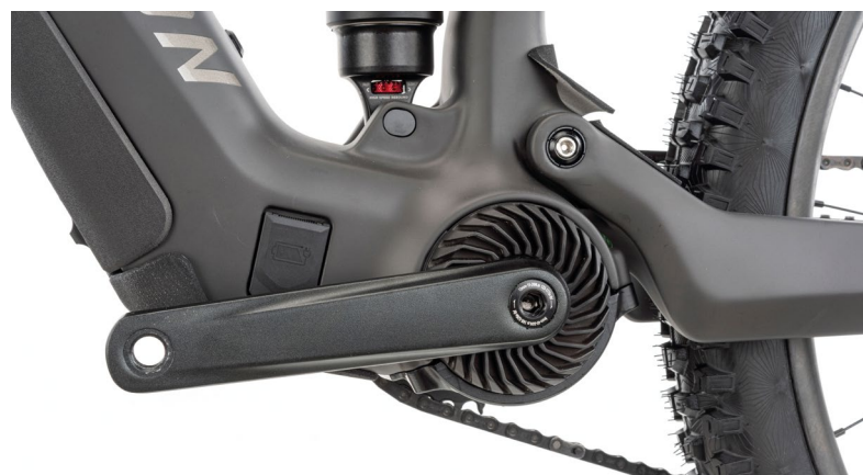
FIGURE 1 The free installation space in the bottom bracket area was utilized: CentriX drive unit from ZF with a diameter of only 88 mm, installed in the Tarok e-mountain bike from Raymon Bicycles (© Raymon Bicycles)
