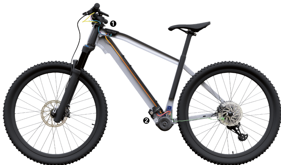
FIGURE 2 The ZF Bike Eco System only requires a single cable routing in the down tube between the core controller ① and the battery terminal ②. All electrical components at the front of the e-bike are connected via the core controller, while all components at the rear are connected via the terminal. This significantly simplifies the installation and retrofitting of components. (neutral bike) (© ZF)
