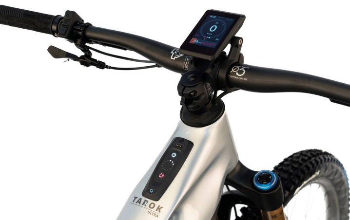
FIGURE 4 View at the control and operating unit of the ZF Bike Eco System with the core controller in the top tube, remote control, and touch display on the handlebars (© Raymon Bicycles)
