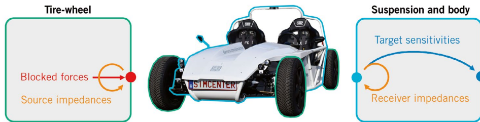
FIGURE 2 C-TPA decomposes the vehicle into independent models for source and receiver components (© Siemens Digital Industries Software)
