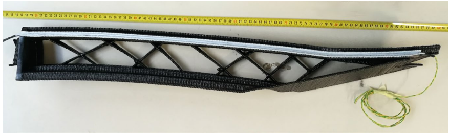
FIGURE 2 Imprinted CAN bus cable into the KTL coated DED-Arc printed A-pillar using APPD (© Inocon)
