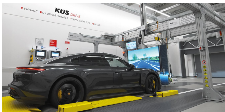
FIGURE 5 ViL on the chassis dynamometer with camera and radar OTA stimulation (© KÜS)
