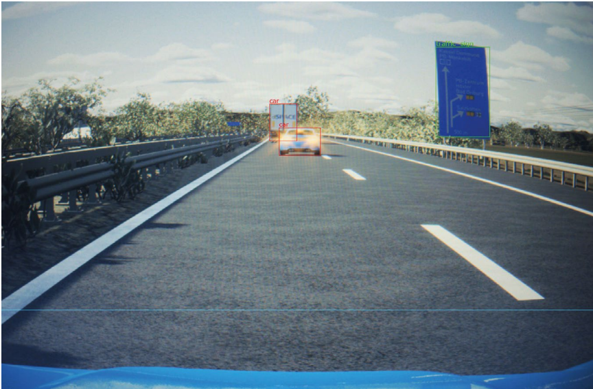
FIGURE 3 Visualization of the camera OTA stimulation (© dSpace)
