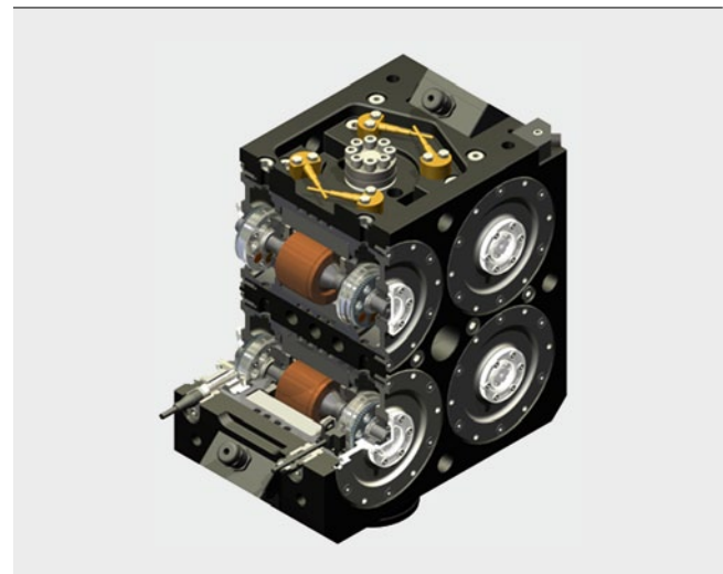
3 The unbalanced mass exciter of the test bench in cross-sectional view
