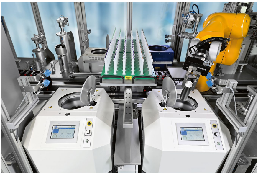
Figure 4 > Vacuum speed mixers enable precise mixing and complete deaeration of high-viscosity formulations, even in small quantities.
