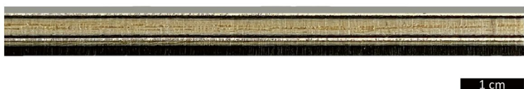
Figure 4 > Cross-section of a multi-material laminate; materials from top to bottom: co-polyamide top sheet, aluminum top chord, neoprene rubber, ash core, neoprene rubber, aluminum bottom chord, ash cut veneer, ultra-high molecular weight polyethylene running surface
