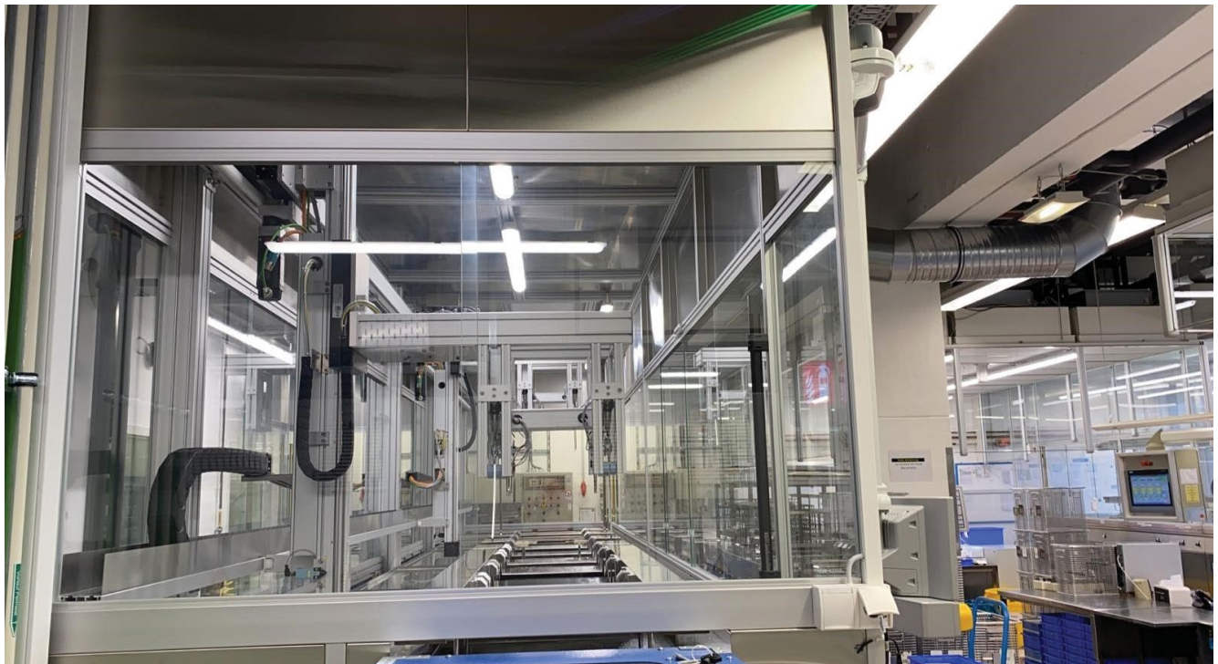
Figure 1 > The various treatment stations of this individually designed ultrasonic ultrafine cleaning system can be flexibly accessed.
