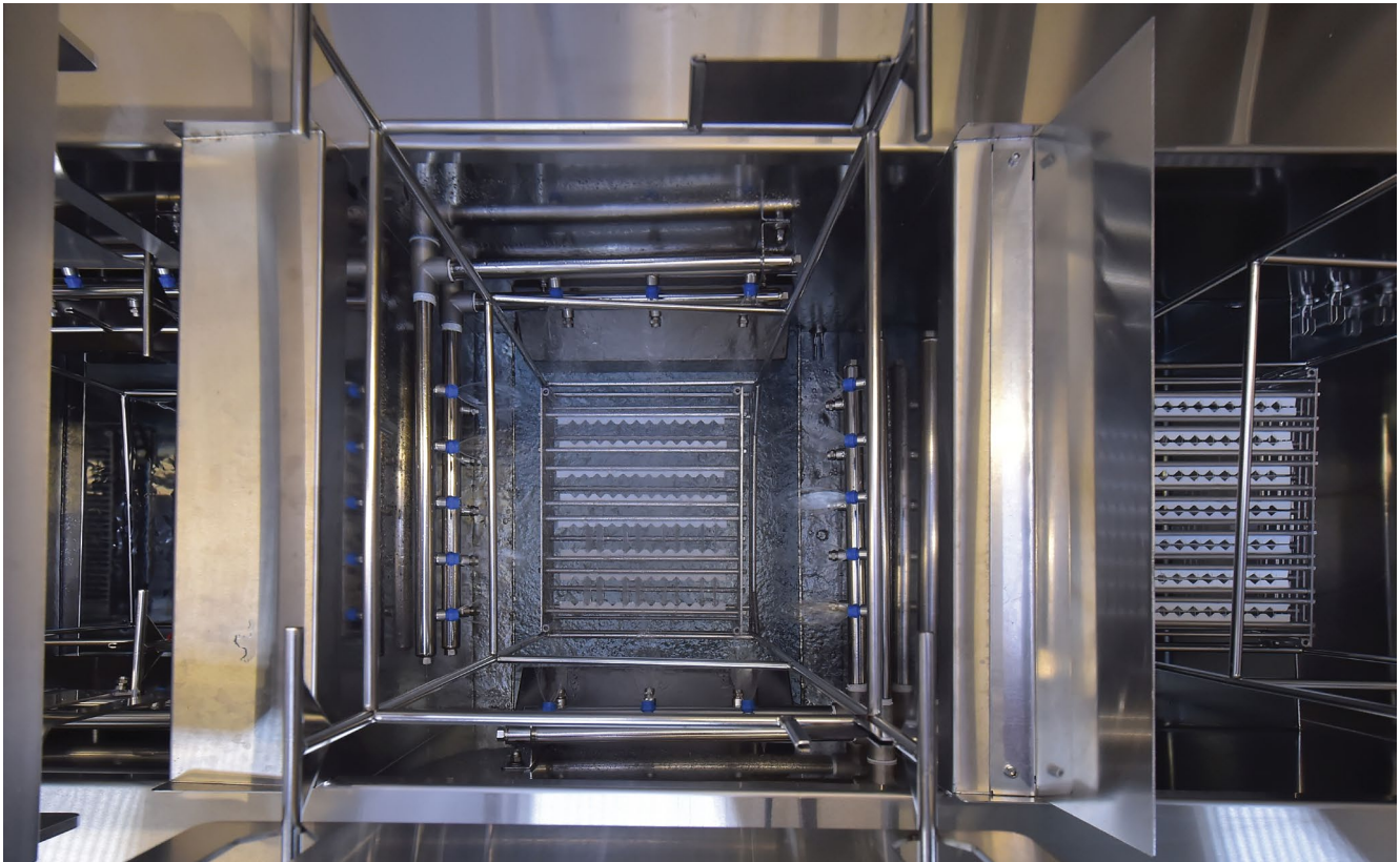
Figure 4 > In the immersion/spray rinse tanks specifically developed for ultrafine cleaning processes, the parts are sprayed off as they exit the bath which enhances the rinsing result.
