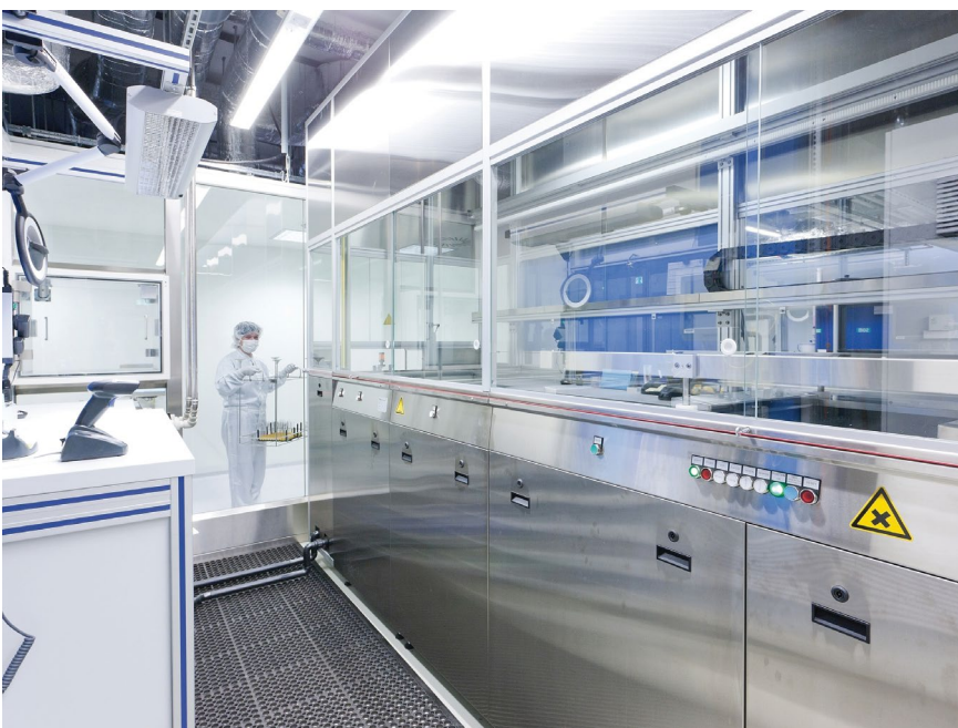
Figure 3 > For integration into clean rooms the ultrasonic ultrafine cleaning systems are fitted out in compliance with the applicable clean room class.
