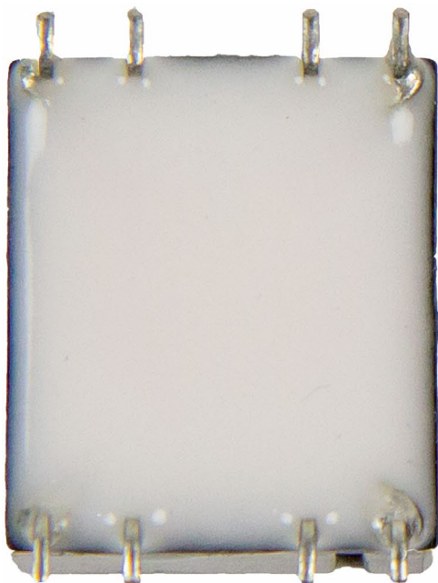
Figure 4 > Encapsulation of a toroidal coil with Novasil S 151 or S 651: The heat generated on the component, for example by current flow, can be reliably dissipated with the aid of thermally conductive potting materials.
