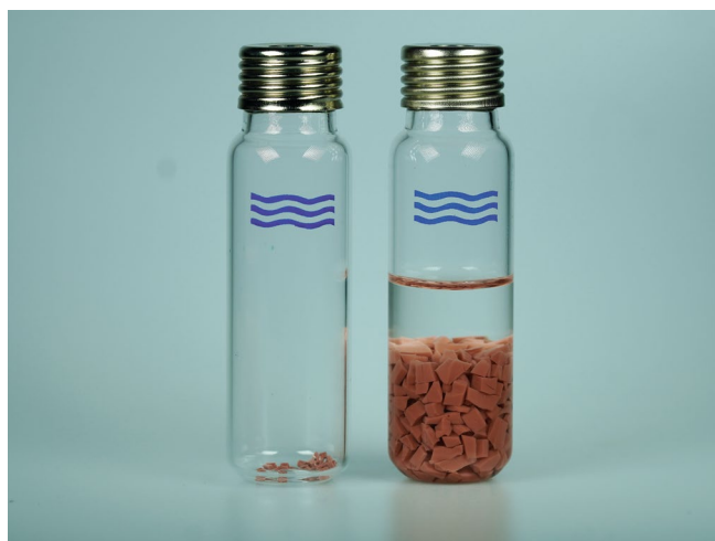
Figure 8 > Sample preparation – right: extraction according to PV 3055 (1 g silicone on 10 ml heptane), left: emission according to PV 3040 under standard conditions (50 mg silicone on 20 ml gas volume)
