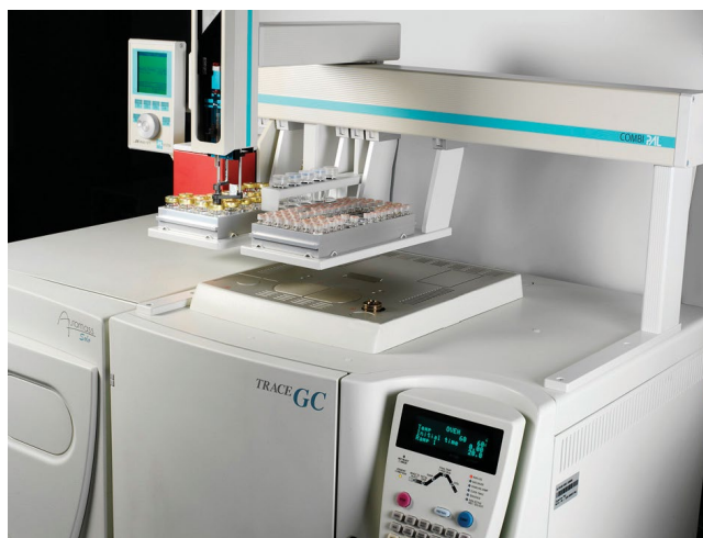
Figure 9 > Typical gas chromatography system with autosampler: oven (left), headspace tray (centre) and tray with vials (right) for liquid injection
