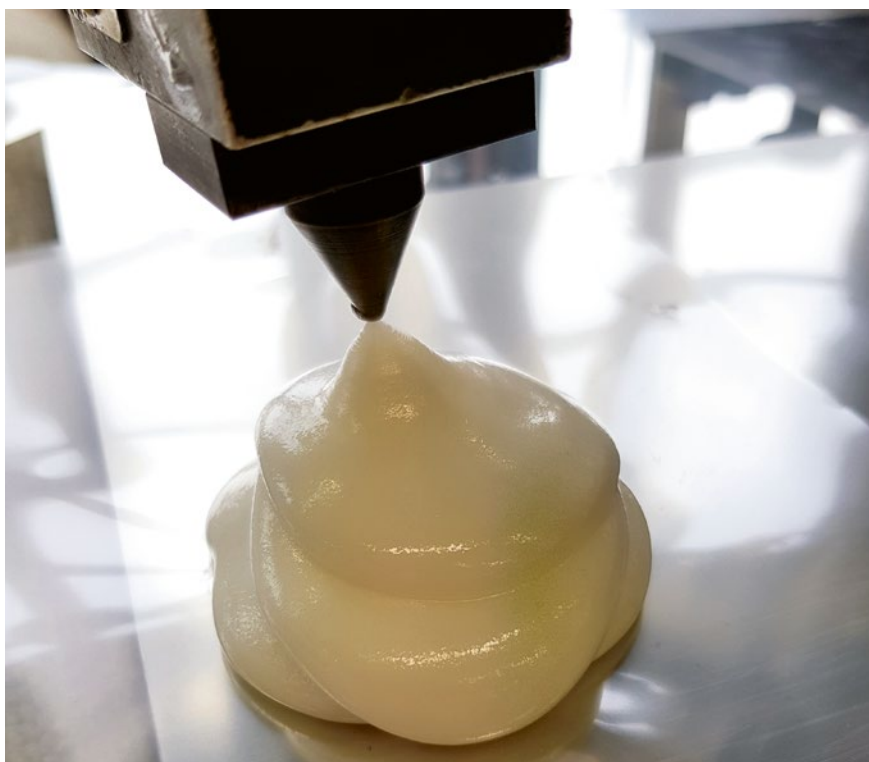
Figure 2 > Hot melt filled with small gas bubbles
