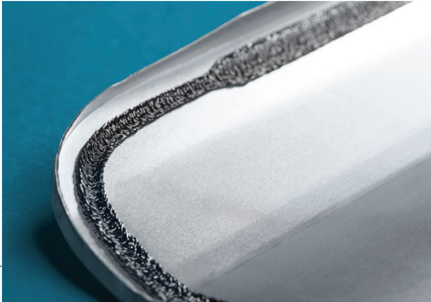
Figure 7 > Application with necking – applied using the swirl method to the outer sheet of a component to be folded. In places where less material is required, especially in curves, the adhesive volume can be systematically adjusted while still maintaining a consistently high application quality.
