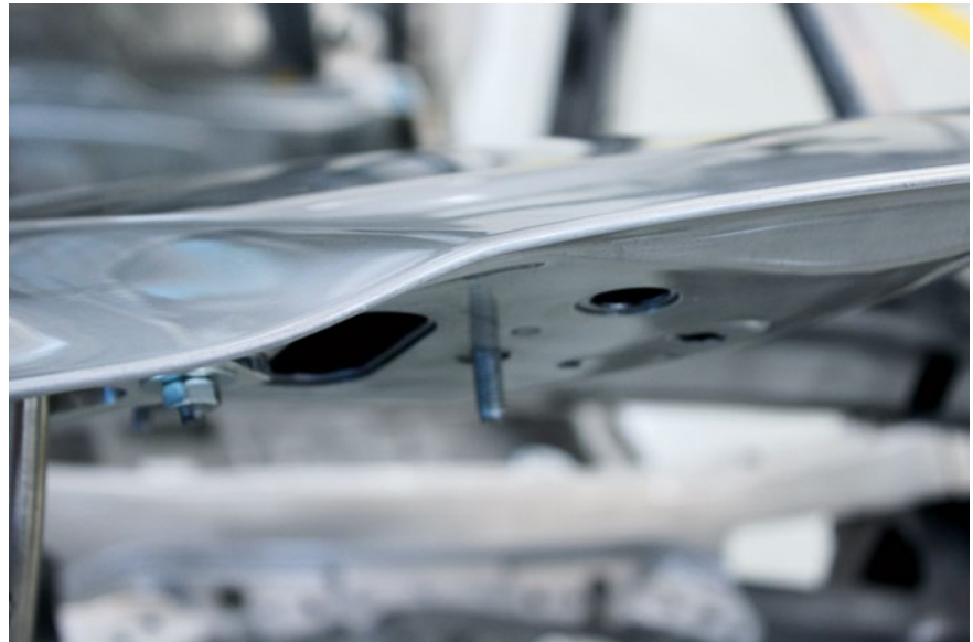
Figure 1 > Motor and trunk lids are typical mounted parts that are folded and bonded during the production process.
