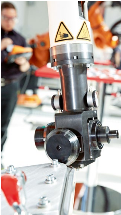
Figure 4 > Roller hem bonding: first step by means of a pre-folding roller. The process achieves a high surface quality, especially for complex component geometries.
