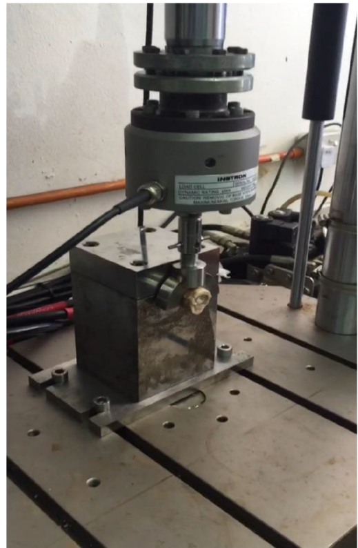
Fig. 2 Instron machine for shear stress test. Shows the shear stress test on the TEHB scaffold using the Instron machine
