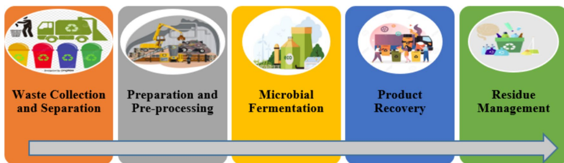
Fig. 8 Flow diagram for the fermentation process of MSW conversion
