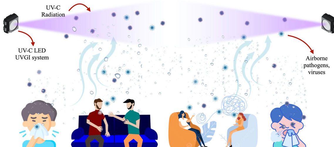
Fig. 6 Schematic representation of UVGI system using LED for disinfecting bioaerosols contamination in an enclosed environment
