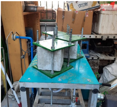
Fig. 4 Water penetration depth test
