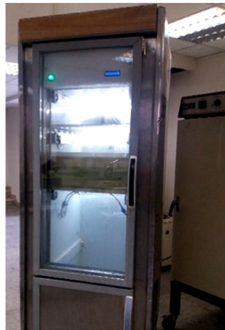
Fig. 5 Carbonation test devices
