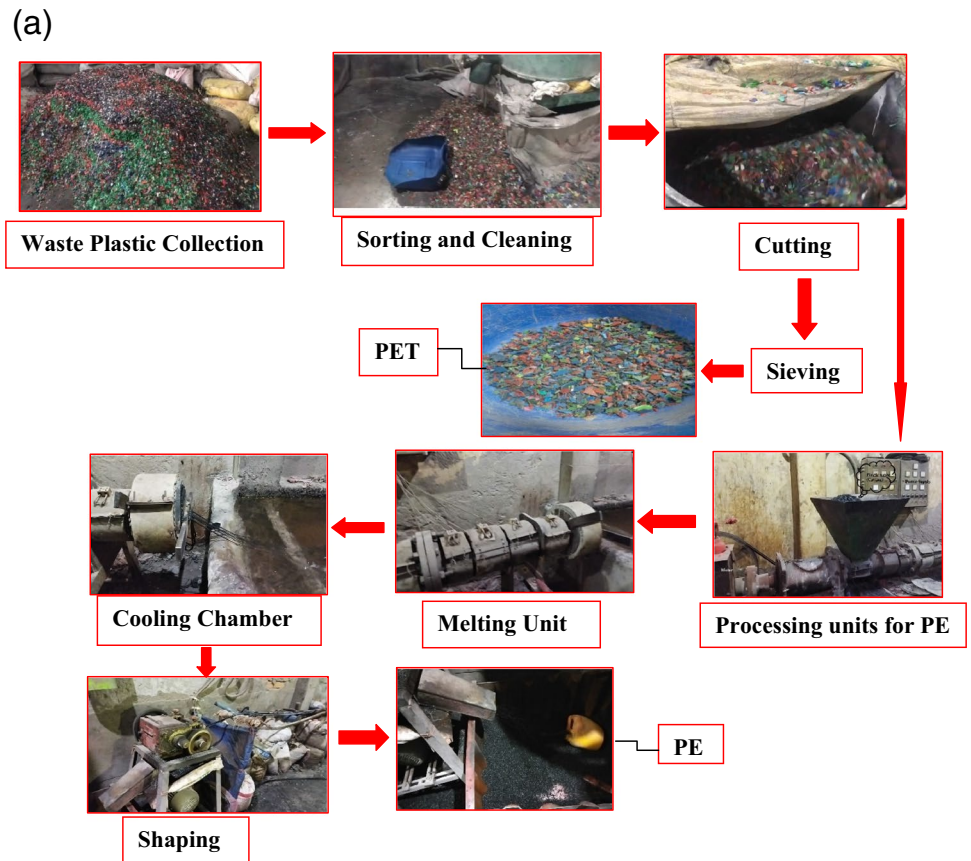
Fig. 1 a The flowchart of processing of PET and PE. b Grading curves of PET- and PE-based and natural aggregates (Source: Shiuly et al.2022)
