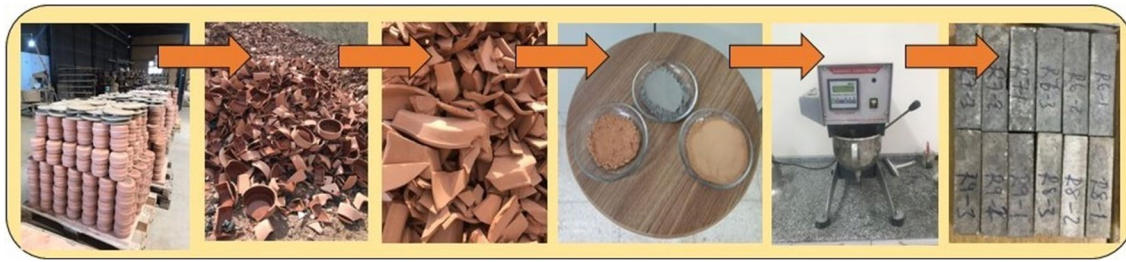
Fig. 2 Preparation of pottery waste and production of mortar from pottery waste and fly ash
