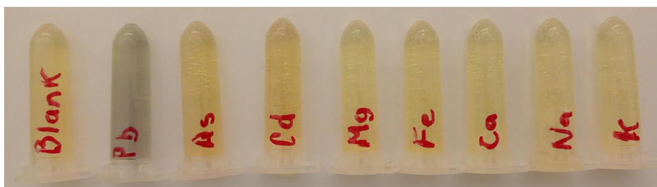
Fig. 3 Photograph of centrifuge tubes containing heavy metal ions, where it is clarified that only the lead solution produces a color change in the original colloidal solution of AgNPs
