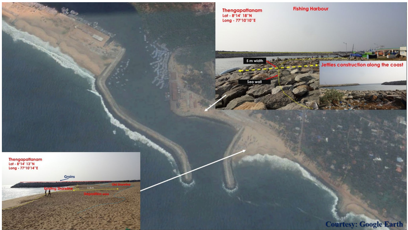
Fig. 9 Modification of the shoreline due to Jetties, Accretion zone on the other side of the construction
