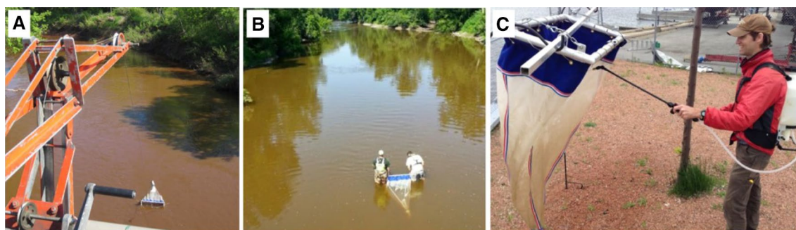
Fig. 5 Different methods adopted for sample collection A. using a bridge crane and B. by wading, and C. using backpack sprayer for washing of particles from the net (Baldwin et al. 2016)
