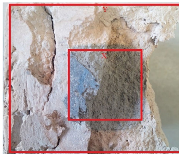
Fig. 7 API Class G cement after immersion test under \text{CO}_2 -saturated brine
