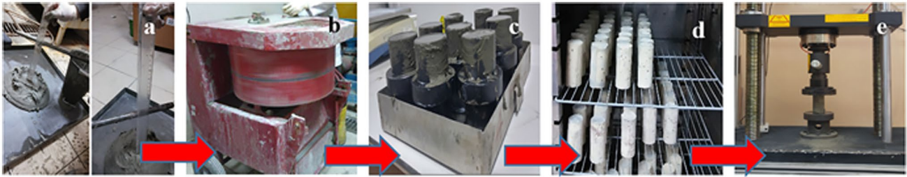
Fig. 2 Main stages of the study (a-slump test, b-mixing, c-molding, d-curing, e-UCS test)
