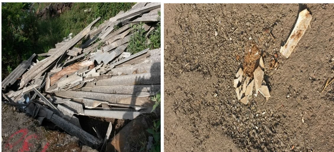
Fig. 2 The asbestos material haphazardly disposed in the campus
