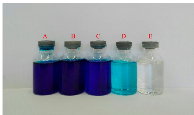
Fig. 5 Fenton’s reaction decolorization, control (a), control with H 2 O 2 (b), EAF (c), Cu/EAF (d), Co/EAF (e)
