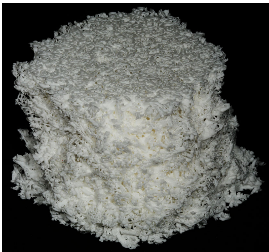
Fig. 9 Physical replica of a Hairy Stalagmite sample created by additive manufacturing (3D-printing) for physical inspection
