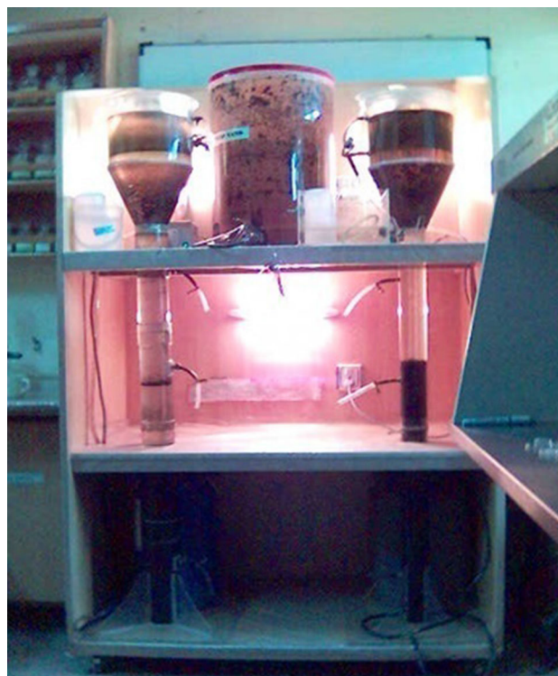
Fig. 2 Photograph of UASB CD and UASB ASDIT reactors during restart-up
