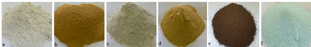
Fig. 1 Photograph of a natural bentonite b Fe-bentonite c natural zeolite d Fe-zeolite e iron filings f ferric sulfate
