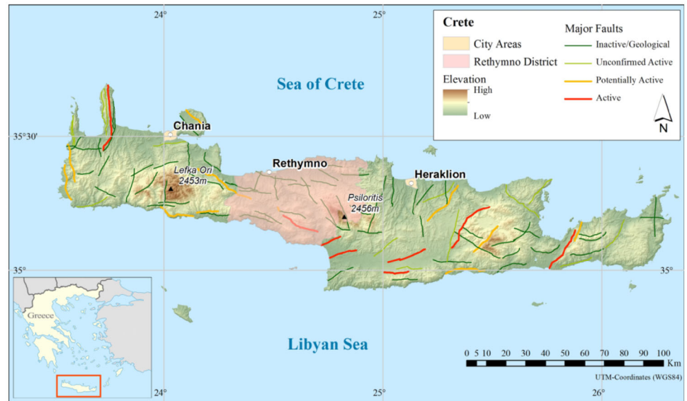
Fig. 3 Topographical map of Crete Island Rethymno District and its surroundings. The DEM (digital elevation model) indicates the variation of the terrain landforms expanding through the whole island. Four different categories of faults have been identified, two of which (active and potential active faults) have been correlated with the mainland seismic activity of the island. Source GeoSat ReSeArch Lab, IMS–FORTH
