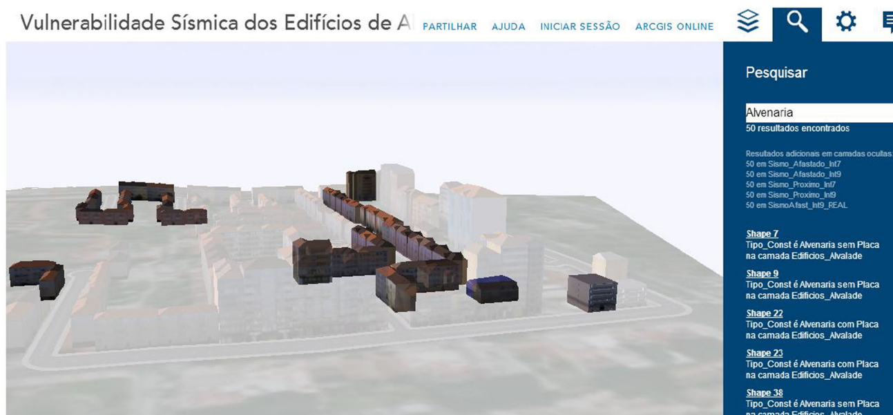
Fig. 3 CityEngine web viewer layout example: result of the query “Type of construction: Masonry—Alvenaria (in Portuguese)” for the pilot area Alvalade; (left) highlighted buildings in 3D scene matching
