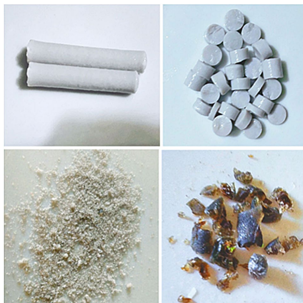
Fig. 1 Highlighting the transformation of SA-g-p(FA-AA)/GO into its final state as adsorbent after undergoing cutting, washing, drying, and grinding stages
