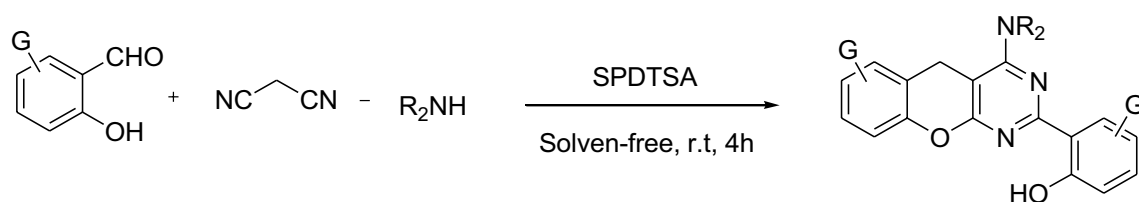
Scheme 32 SPDTSA catalyzes one-pot synthesis of benzopyrano[2,3- d ]pyrimidines
