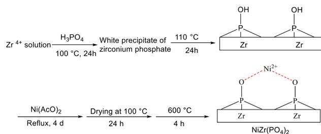
**Scheme 1** Procedure for the preparation of ZPNi
