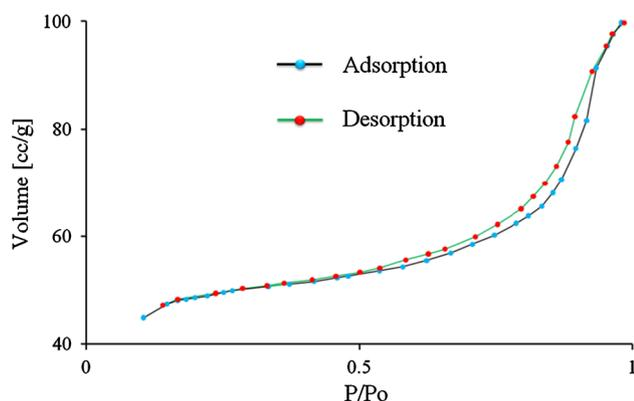
**Fig. 2** N<sub>2</sub> adsorption–desorption isotherm of ZPNi
