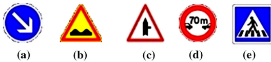
Fig. 1 Traffic signs types: a mandatory sign, b temporary sign, c warning sign, d prohibition sign, e reservation sign
