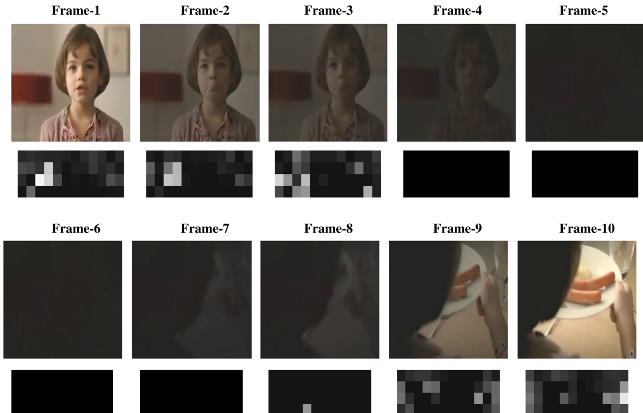
Fig. 9 A set of ten consecutive frames of a fade out/in transition extracted from advertising video in dataset-2 where the SIFT-PDH of each frame shows clearly the shot boundaries (frame-4 presents end of the current shot _i and frame-8 presents start of the consecutive shot _{i+1} )
