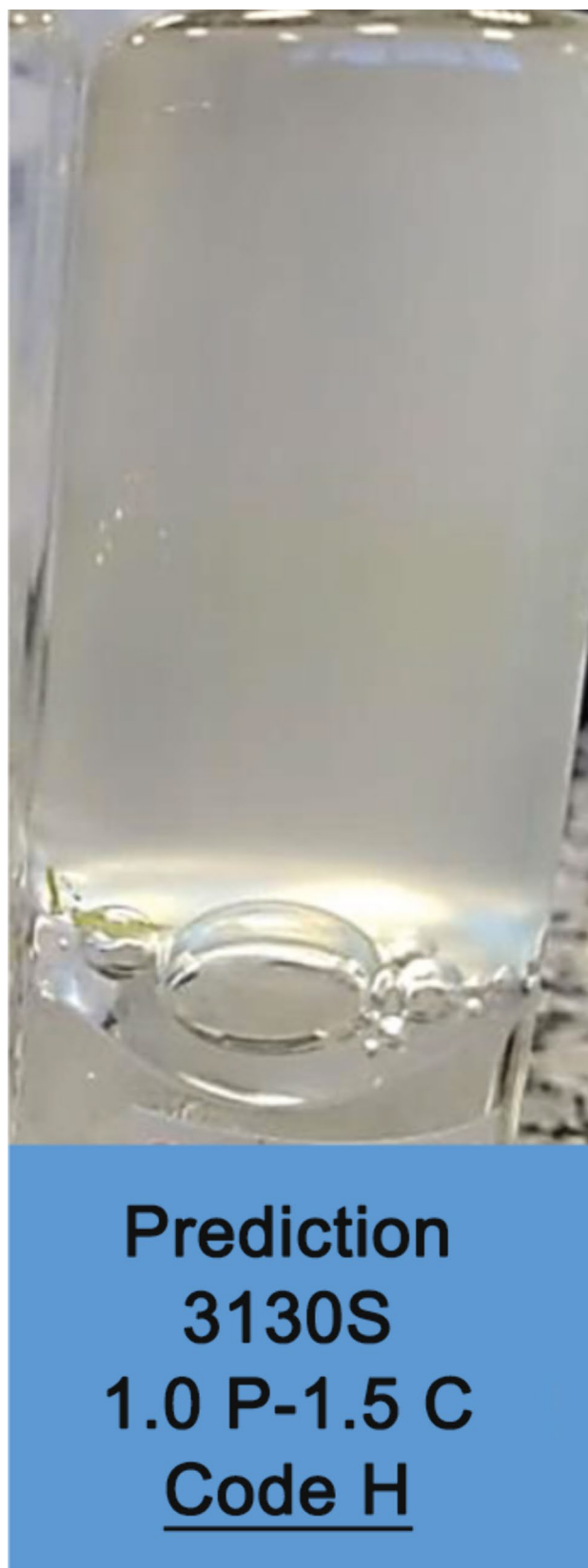
Fig. 2 Visual appearance of the prediction gel created based on the statistical results. Prediction: 1.0P–1.5C – H code
